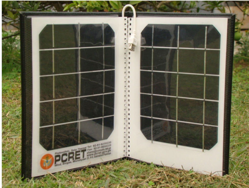
Figure 3: Solar Mobile Charger developed by PCRET
