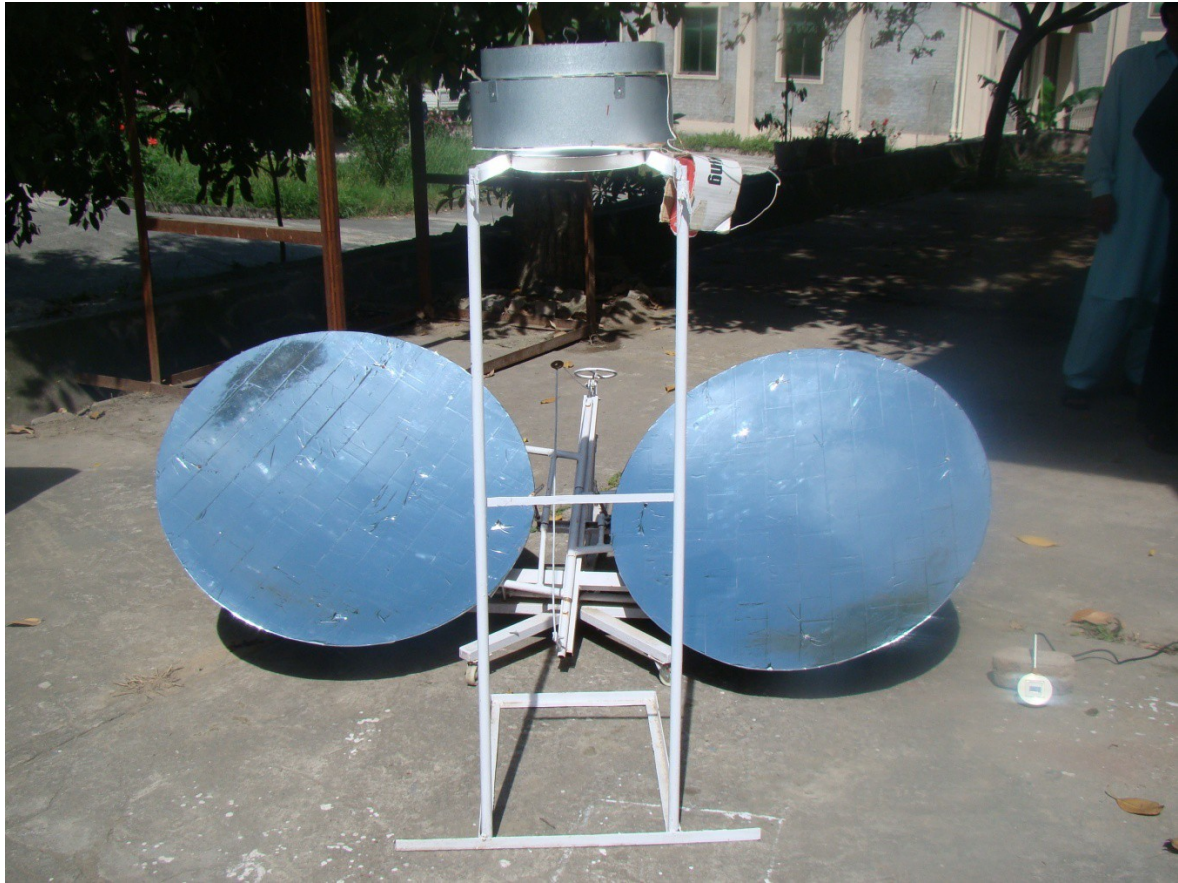
Figure -1: New Type of dual Parabolic Reflector Solar Cookers
