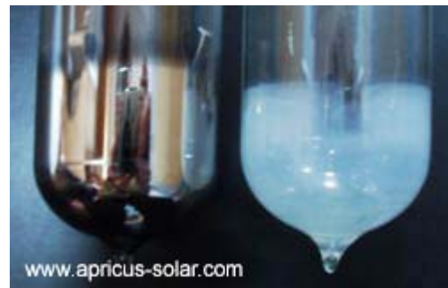
Left Tube = Vacuum Present Right Tube = Faulty
