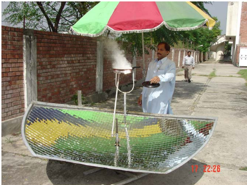
Parabolic type solar cooker (Reflecting material: aluminium foil Dish material: fibreglass and cement Stand made of angle iron)
