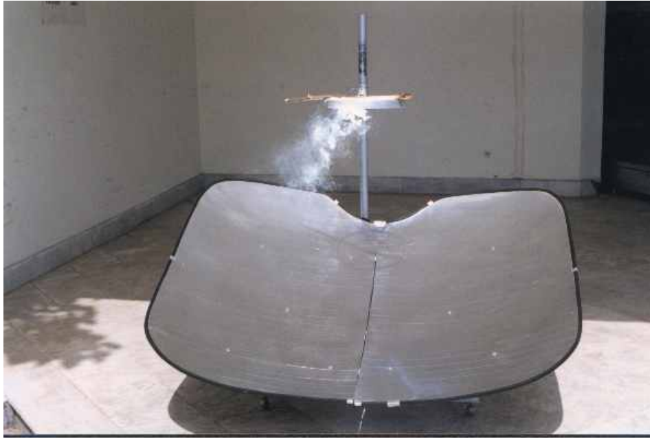
Parabolic type solar cooker (Reflecting material: aluminium foil Dish material: fibreglass and cement Stand made of angle iron)
