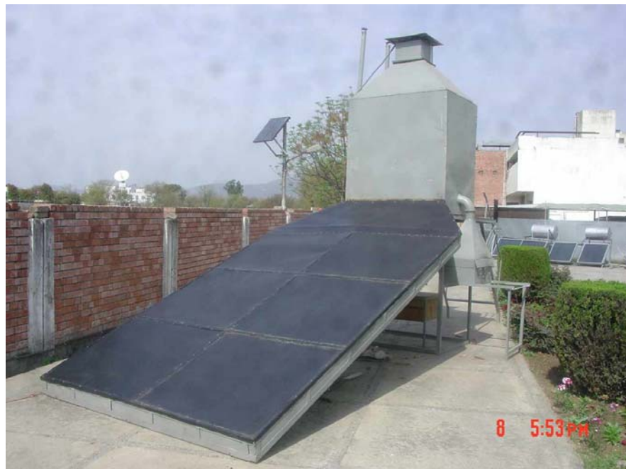
Unglazed type transpired collector type hybrid (Solar-biomass) dryer 150 kilogram loading capacity
