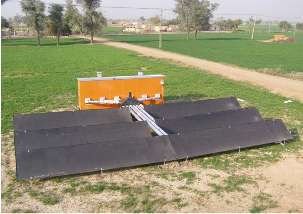
Unglazed collector type hybrid (solar-biomass) Dryer 500 kilogram loading capacity
