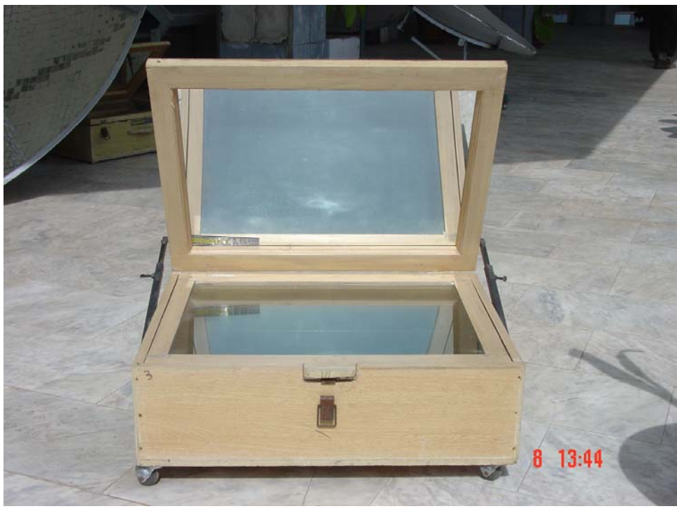
Box type Solar (Body: wooden and Iron sheet Reflecting material: Ordinary glass and transparent glass Heat retaining material: glass or rock wool)
